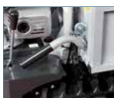
Manual dump with automatic locking system.
